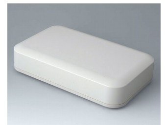
A9481107 EVOTEC 250, Ausf. I ASA+PC-FR (UL 94 V-0) grauweiß RAL 9002 250x155x54mm IP 65 opt., IP 40
