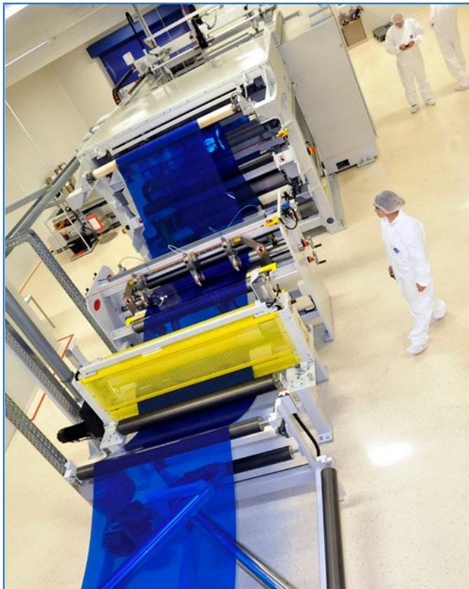
**Tekni-Plex produces its multilayer coextrusions in an ISO 7 cleanroom.**
