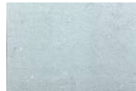
Superfinish-Treatment (magnification x 2000)
