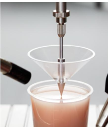
Penetration Test of ELASTOSIL® P grades
