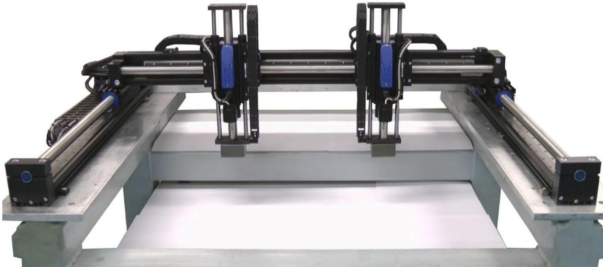
Figure 5: X, YY, ZZ multi-axis system with two independently moving Y/Z axes
