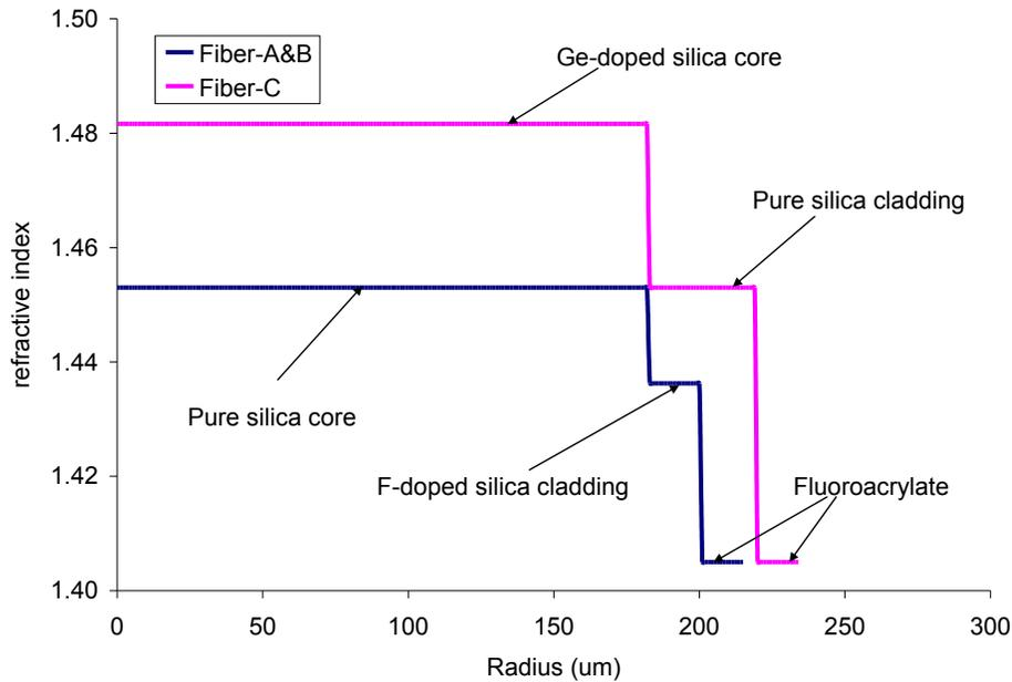
**Figure 2 Index profile of Sample-A, B and C**
