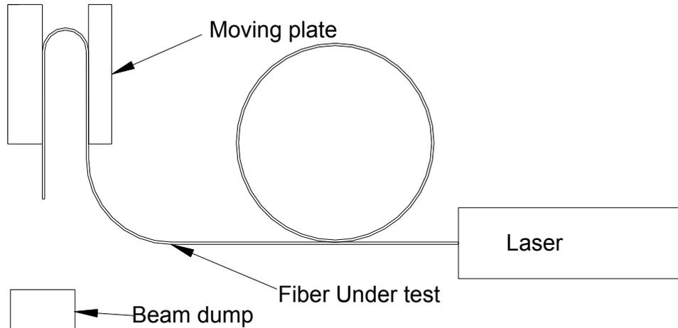
**Figure 1 Experimental setup, 100 W of laser power is launched into the fiber when bent, excess fiber was looped into a diameter of 20 cm**
