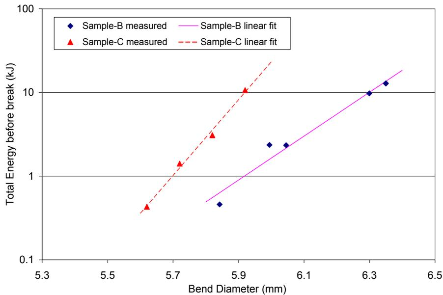
**Figure 4 bend diameter vs. total transmitted energy**
