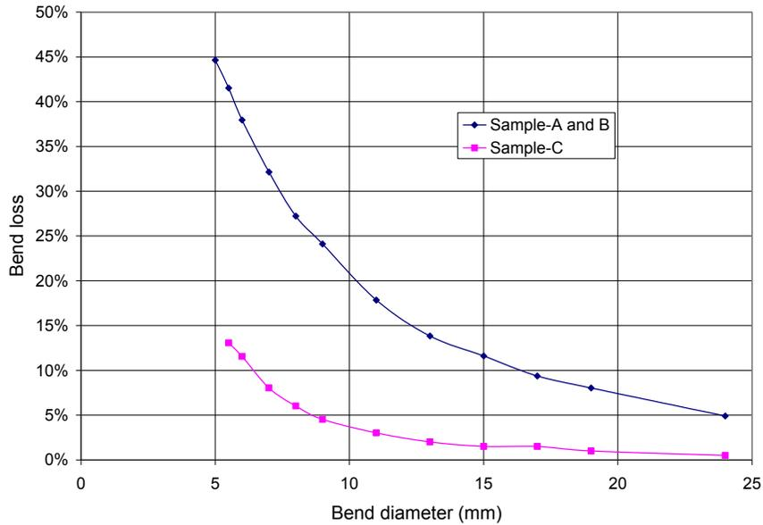
**Figure 5 Bend loss of Sample-A, B and C at 2.1  $\mu\text{m}$  with 0.22 NA launching**
