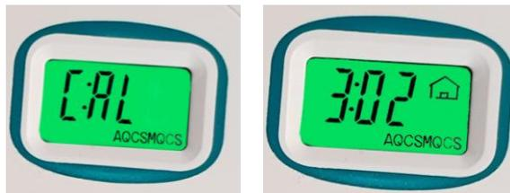
As an alternative, it is possible to use the **MQCS (Manual Quick Calibration System)** which allows the device to immediately stabilize its temperature to the room temperature in just 3 seconds.
