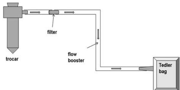
**FIGURE 3.** Schematic diagram of the smoke collecting system.
