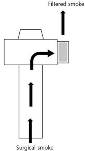
**FIGURE 2.** Schematic diagram of the built-in-filter trocar. The arrows indicate the flow of surgical smoke.
