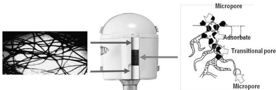
FIGURE 5. The filter is made of 2 layers of processed and refined charcoal (left arrow). Each layer has 1200 m<sup>2</sup>/g surface to absorb a large amount of smoke. The space between the 2 charcoal layers (right arrow) is occupied by innumerable 1 to 50  $\mu\text{m}$  micropores designed to trap liquid and aerosolized substances.
