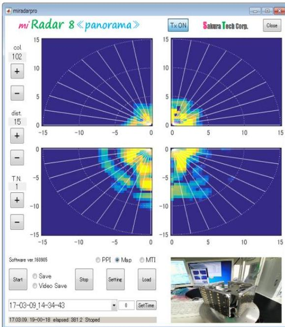
Evaluation software (Professional Version) is a Matlab execution file that controls coordinating operation for a maximum of four miRadar8 and displays processing results.
