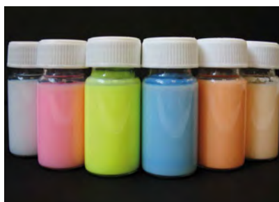
PMMA-submicron beads with tuneable spectral properties and high fluorescence intensity
