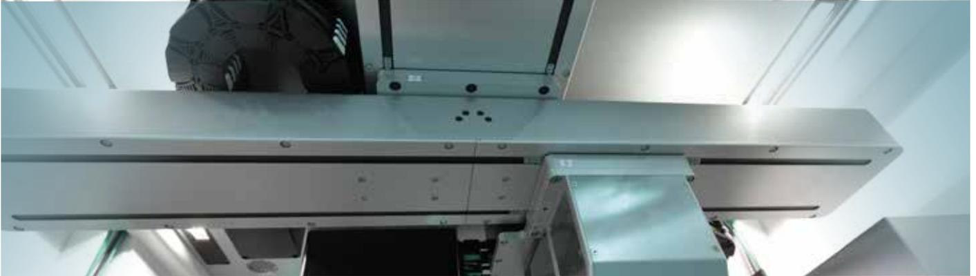
Precise kinematics: Closed linear axes with accuracy of 10  $\mu\text{m}$  @ 6 sigma
